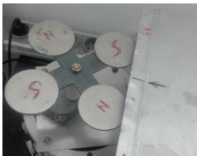
Figure 2: Photo of VLF magnetic field set up.
