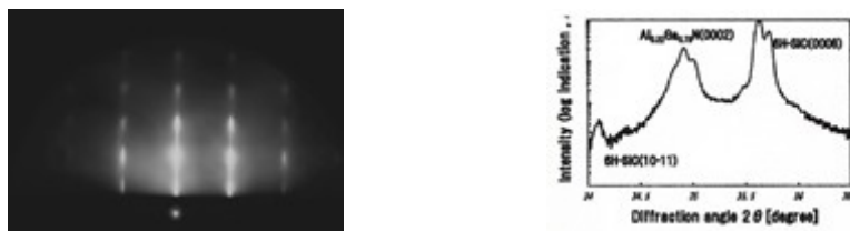
Fig.2. RHEED pattern and X–ray diffraction pattern of AlGaN/AlN films on the surface–treated 6H–SiC(0001)
